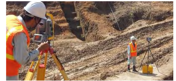
Trimble S6とTrimble TX5の併用
